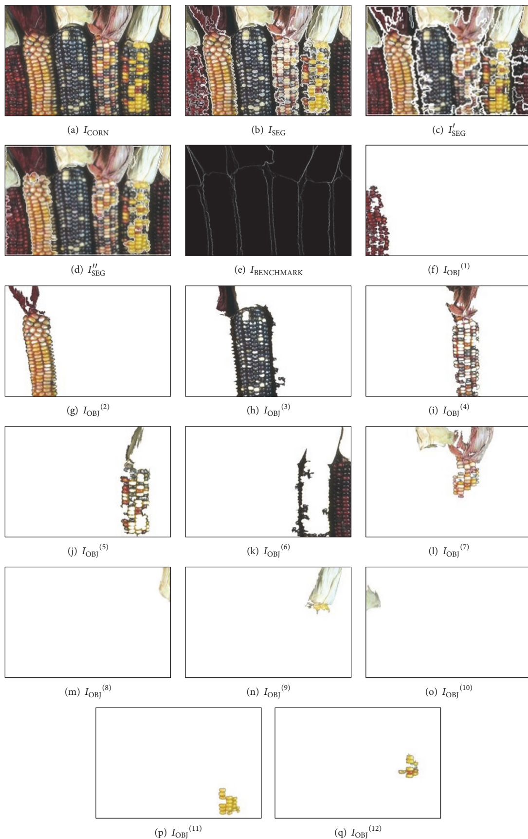
FIGURE 7: Source image, I_{\text{CORN}} ; segmented images in the RGB, HSV, and YUV space, I_{\text{SEG}} , I'_{\text{SEG}} ; and I''_{\text{SEG}} ; manually made benchmark, I_{\text{BENCHMARK}} ; and partitioned objects in the RGB space, I_{\text{OBJ}}^{(i)} .
