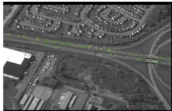
Figure 2: Image of vehicle detection in WAMI data.
